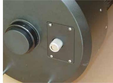
There are two different types of focus knobs on the C-9.25. If you have the one with the rubber focusing knob, remove the cover plate and then pull the rubber knob from the focusing nut. Be patient, these can sometimes be stuck and may take some coaxing to remove them. The rest of the instructions are the same for both models. If you have any difficulty feel free to contact us.
