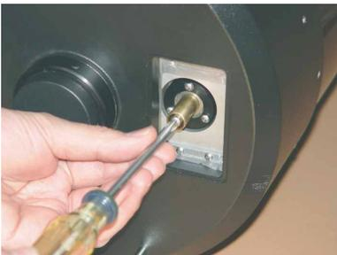
**1.d.** Remove the Phillips screw from the focusing stem as shown.
