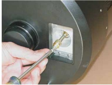
2.b. Reattach the Phillips screw onto the focusing stem as shown. **IMPORTANT:** This screw secures the mirror assembly and must be reattached to prevent the mirror from falling forward if the focusing knob is unscrewed all the way.
