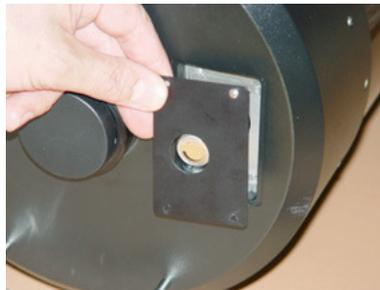
**1.b.** Remove the cover plate as shown. You will replace it with the new one that is supplied with the Micro Kit.
