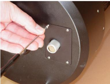
**1.a.** Place the telescope on a towel or a clean work surface and remove the (4) Phillips screws as shown.
