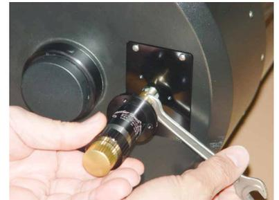
2.f. Hold the unit as shown on the black coarse focusing knob and tighten the nut onto the Micro with an open end wrench.
