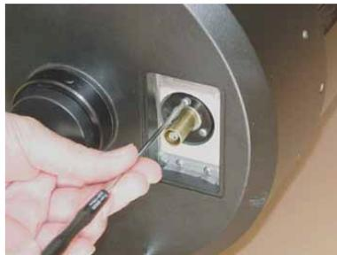
**1.e.** Loosen and remove the (3) Phillips screws that hold the bearing cover housing.
