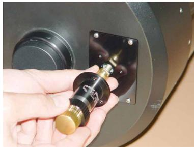
2.e. Screw the focusing nut onto the end of the Feather Touch Micro until snug.
